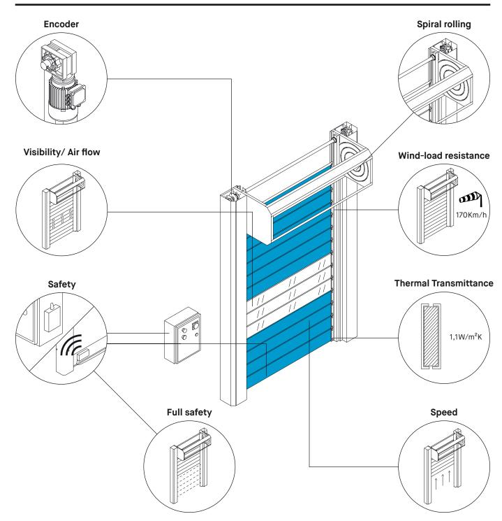
High Performance Door with insulated rigid panels leaf, vertical rolling in patented spiral guides, built in high density polyethylene, to assure smooth and noiseless high speed motion.
